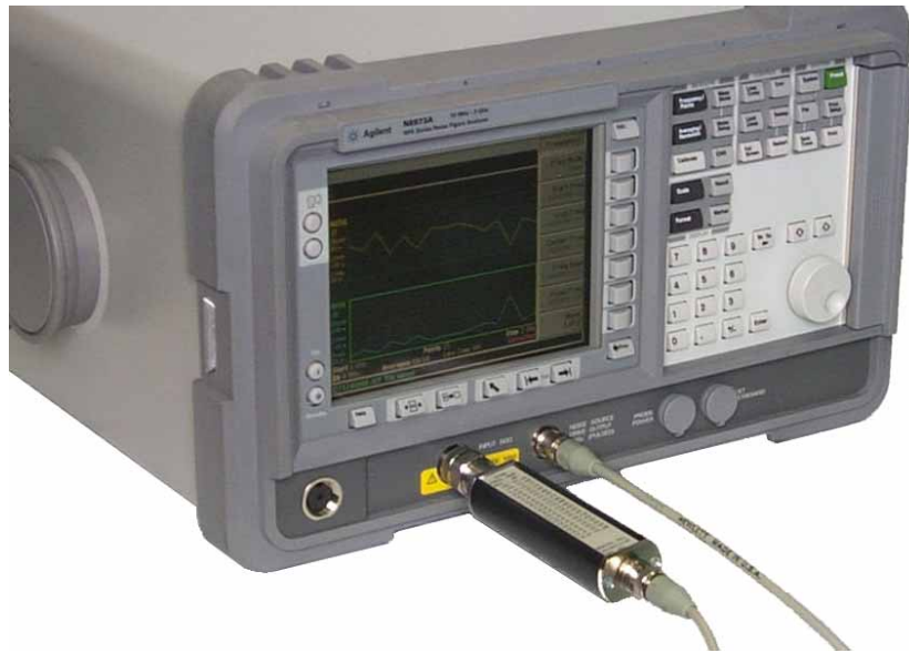
Figure 1-1 NFA with a Normal Noise Source connected
